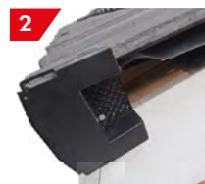
Fix the Eaves Closure to the end of the fascia board or brickwork or additional timber as required to accommodate a suitable fix. Any additional timber should be securely fixed to the rafters.
